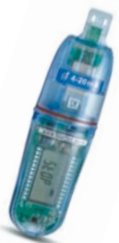
External 4 to 20 mA input LITE5032L-4/20
